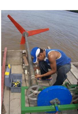
Figure 3: A robust and simple design was developed for remote locations. A simple permanent magnet generator was designed (painted blue). Photo: Soluciones Prácticas.
